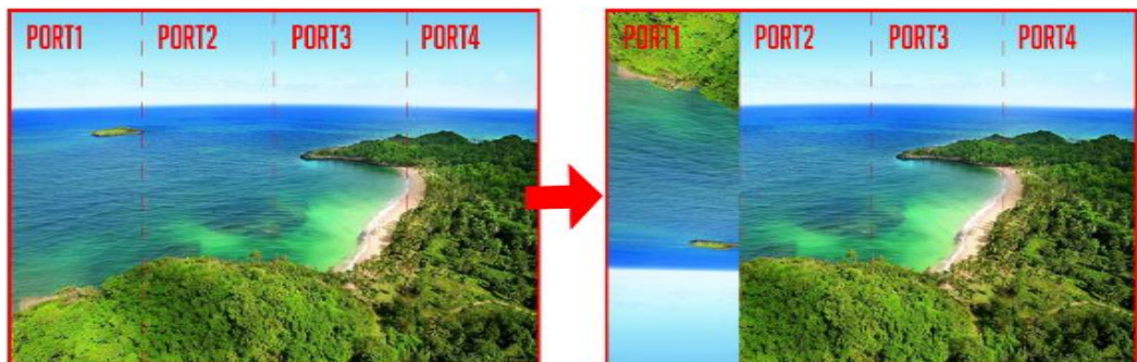
Figure 7-17 Top-bottom mirroring of the image loaded by Ethernet port 1
